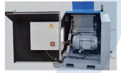
To minimize the needed floor space and make the machine easy to move the control cabinet is integrated into the machines soundproof housing.
