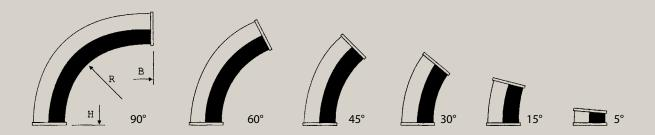
Increasing demands for durability and strength is the reason for introducing the new OKX range. Especially the bends are exposed to wear in pneumatic conveying systems. Therefore Kongskilde is introducing the OKX 160 bends, which have a considerably higher wear resistance and therefore a longer lifetime compared to standard bends.
