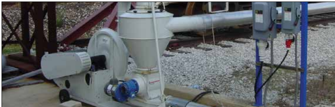
SUC 200 E suction blower used for emptying hopper rail cars with plastic pellets and conveying the pellets into storage silos.
