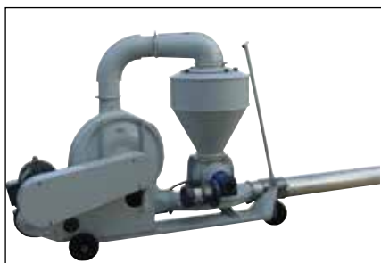
Suction blower used for conveying from and to multiple destinations. This SUC-E is trolley mounted and easy to move.
