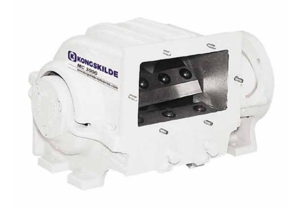
To obtain variable cutting speed, the cutter can be operated via an electrical frequency control - min. RPM 600.
